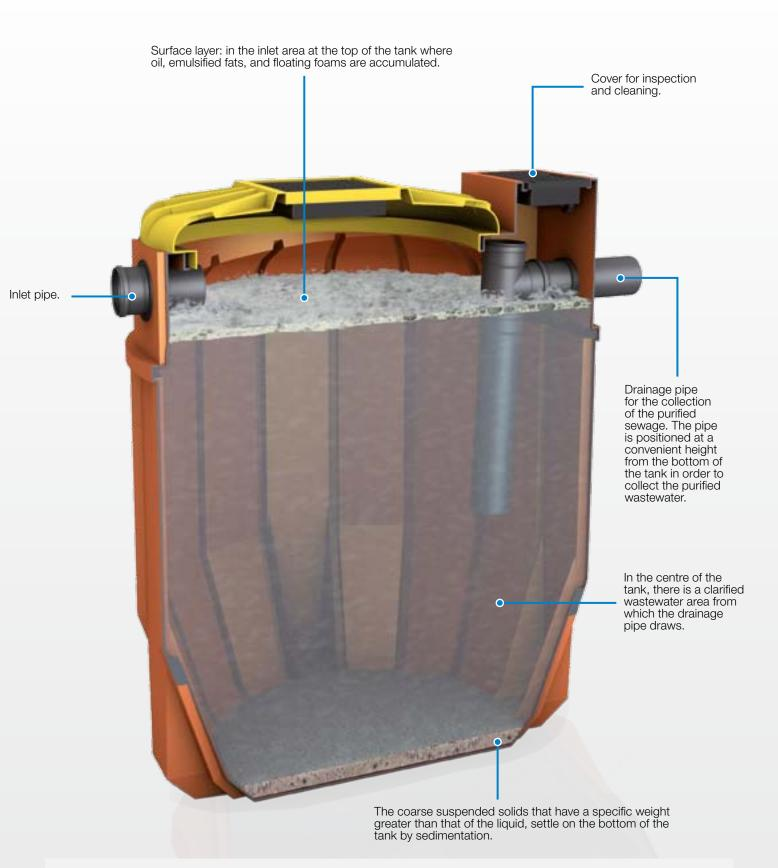
Grease removal unit under the sink
