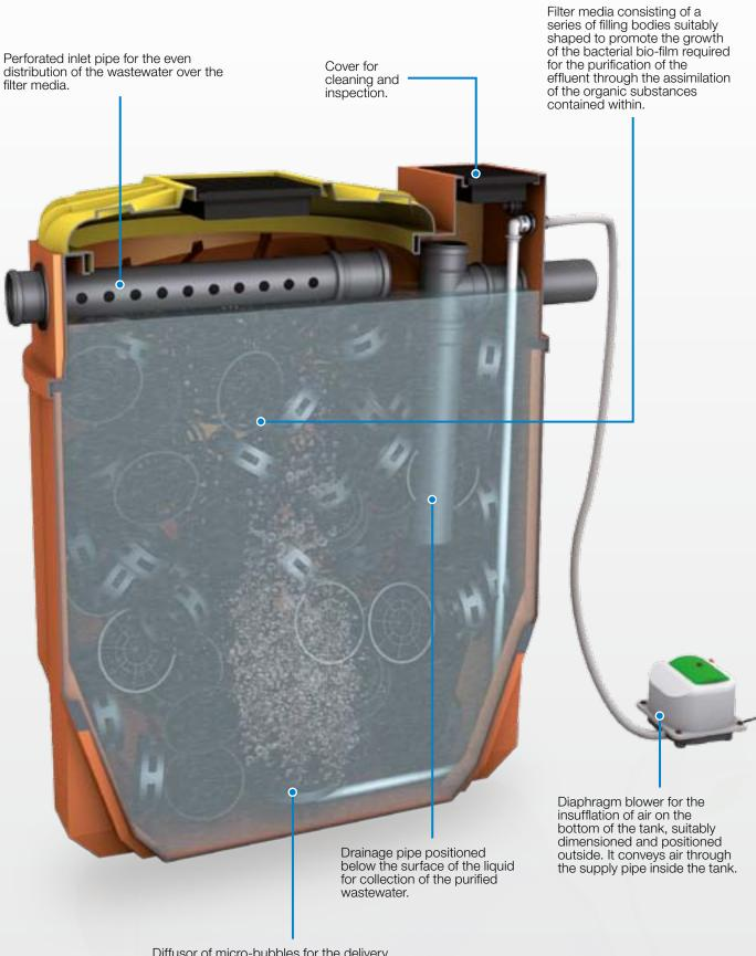
Diffusor of micro-bubbles for the delivery of blown air below the filter media. It consists of a plastic plate (EPDM) with high deformability and a high transfer efficiency of oxygen to the liquid mass.
