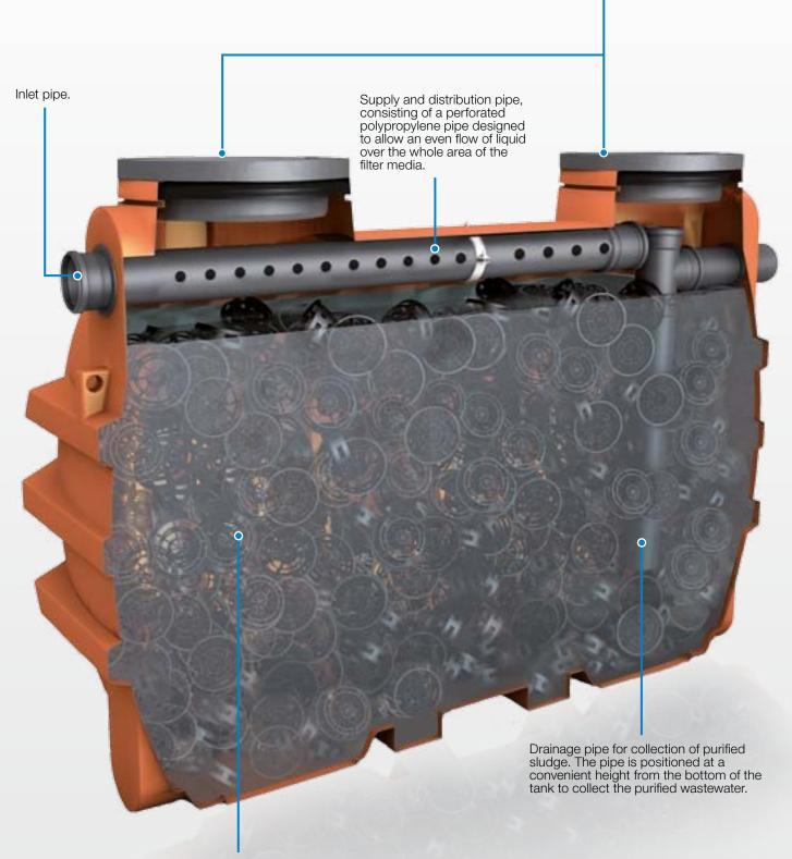
Filtering mass consisting of a series of filter media, suitably shaped, made of plastic. The filter media are plastic and are designed to promote the growth of a bacterial film on the surface required for the purification of the water.
